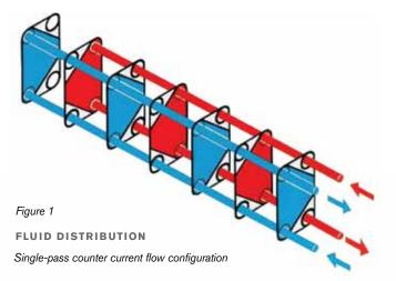
APV plate heat exchangers can be used in a variety of different configurations.
